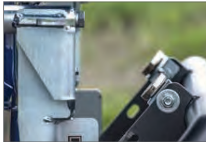
MagLatch™ secures grille guard upright with rare-earth magnets
