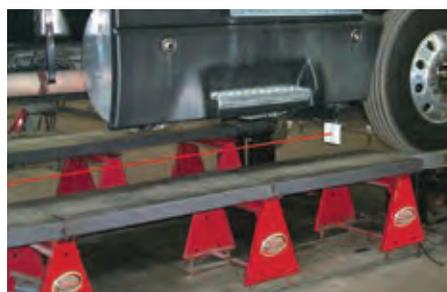
The laser beam is aimed forward in a line identical to the axle's thrust line and strikes the front target, which measures the amount of axle error from the centerline of the vehicle.
