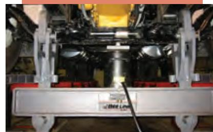
*To correct caster and camber on trucks, Bee Line developed the "Floating Beam System."*
