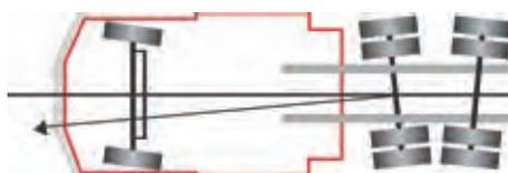
Tracking refers to rear axles. They must be parallel to each other and perpendicular to the center line. If not, the driver must compensate by holding the steering wheel off-center, causing rapid and irregular steer tire wear.
