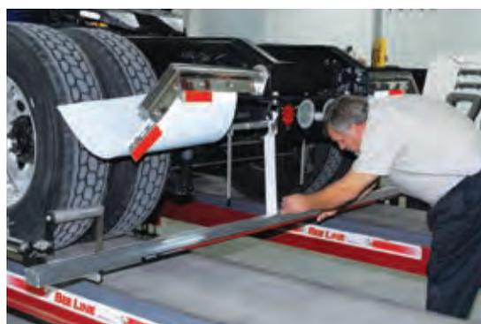
The proven 22000 lets you accurately position your rear axles perpendicular to the vehicle's centerline, allowing the wheels to travel in a straight line.
