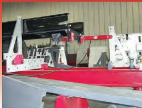
This diamond correction set up utilizes the force of a pull ram to bring the frame rails even with each other.
