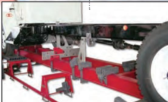
Our Frame Press hydraulically raises to bring the correction tooling to the truck. Runway sections are removed to allow easy access at a comfortable working height.
