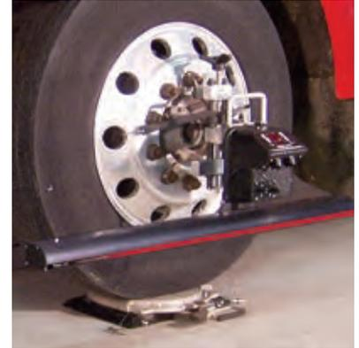
tracking and set the toe in any bay of your shop. If more extensive misalignment conditions are detected or if parts need to be replaced, the truck can be sent out to a facility with a complete Bee Line Alignment system for these corrections. Our On The Floor Alignment configuration is a fast, easy and less expensive way to make sure your trucks are performing at optimum efficiency.
