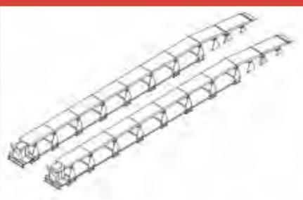
**AA 7D2 WITH AR 330C - 7-Section above ground wheel alignment machine with double approaches (43' 6" long x 24" high) (1325.88 cm long x 60.96 cm high)**
