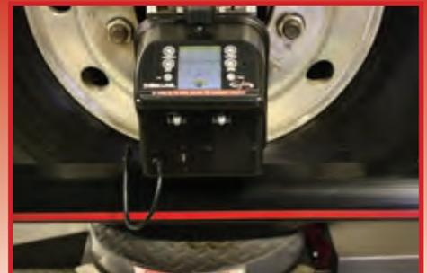
Interactive alignment heads are a "workstation" for the technician. Wireless up to 1,000 feet.
