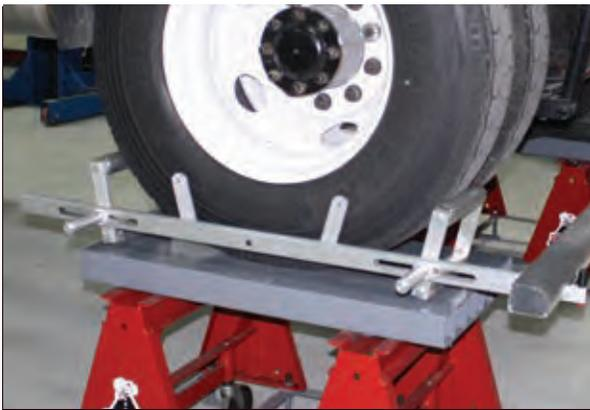
The wheel cradles feature rack and pinion frame gauges that assure accuracy when determining the axle center.
