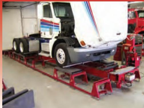
Frame gauging and equipment set up is done at a convenient height. Runways can be removed to allow easy access.
