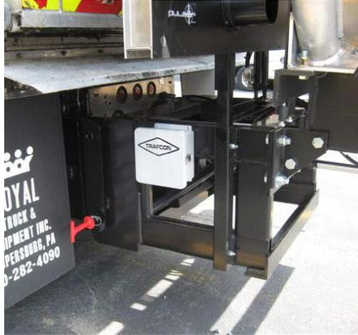
Fast-Trak w/30" Extension and Vertical Arrowboard Lift
