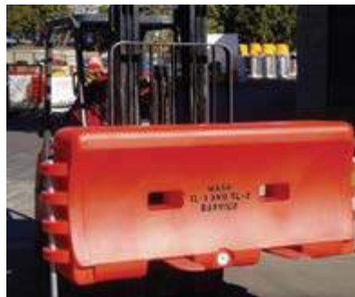
Water-Cable Barrier can be easily moved using a forklift or pallet jack
