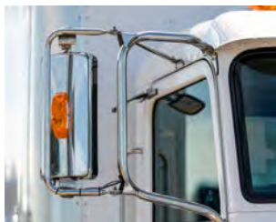
Marker light provides additional safety by signaling other drivers (select models)
