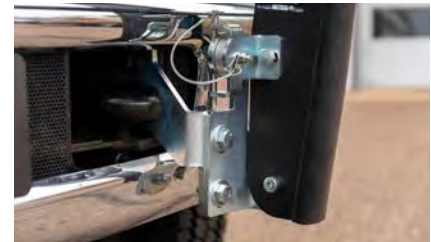
Frame-mounted uprights for improved rigidity and structural support
