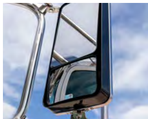
Motorized glass angles vertically and horizontally with 4-way actuator
