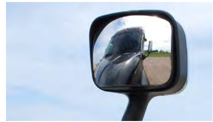
Convex glass helps eliminate blind spots for safer maneuvering
