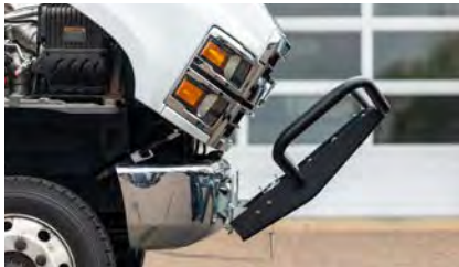
Tilting mechanism allows hoods to be opened safely with full clearance
