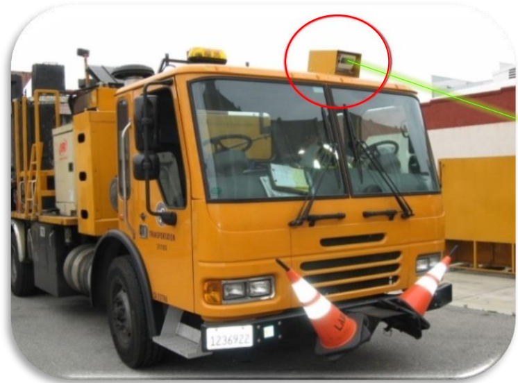
GL3000P-Using centerline as reference for laser guidance
